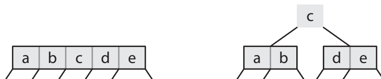
Figure 2.2.: During the insertion, a node split makes one key redundant which can then be used as the splitting key.
