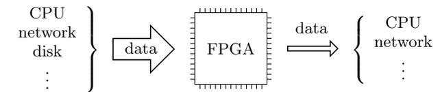
The task of the FPGA here is to act as an early *filter* or *aggregator*. Located close to the data source, the FPGA often significantly reduces the volume of the data before a general-purpose CPU performs more complex high-level operations.
